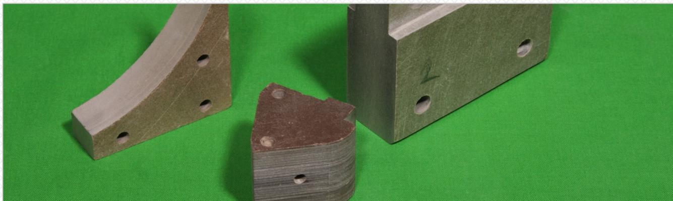
**TENMAT** ARCLEX has been developed as a quality machinable glass bonded mica. It is resilient against high power electric arcs and is widely used in arc chutes for both static (e.g. power stations) and transport applications.
